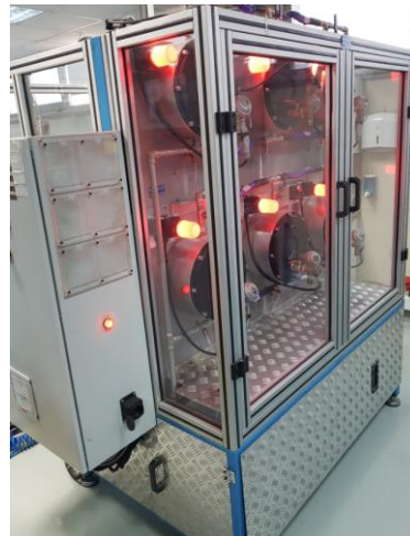
Functional Test Machine for Washing Machines
