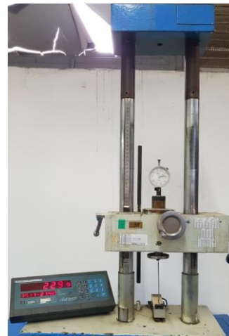
Spring Load Measurement Device
