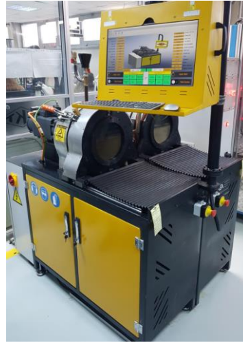
Mud / Dust Functional Test Device
